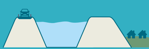
Embankments and walls hold rivers within their banks during high flow
