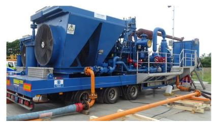
Mobile recompression equipment Source: National Gas Transmission, PMC
