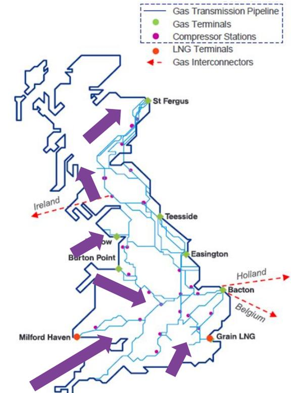
Natural gas ‘pushed’ back to the network injection points, to facilitate an efficient deenergising of the network and decommissioning.
