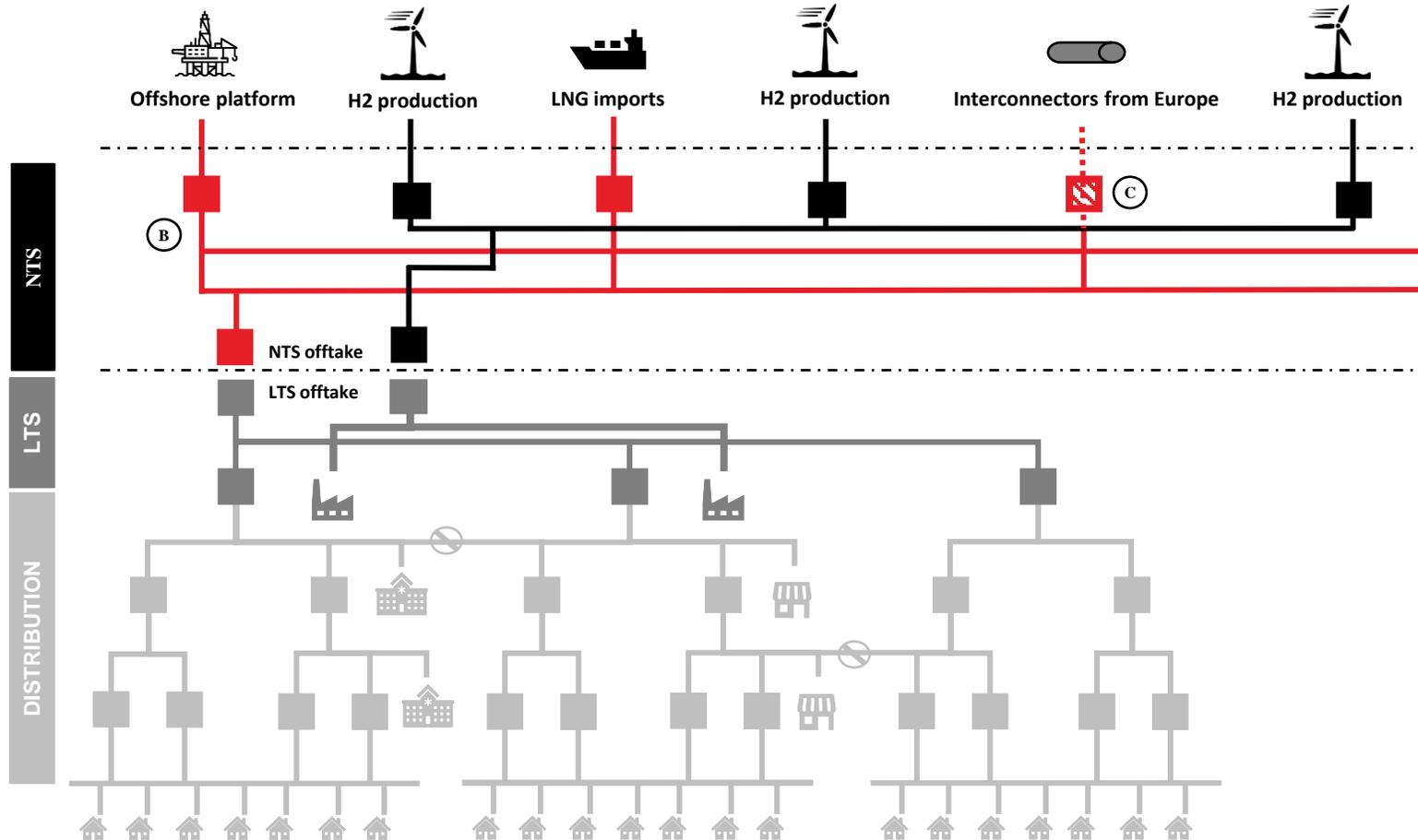
**5b** With significantly reduced natural gas demand the NTS can be deenergised and mothballed.
