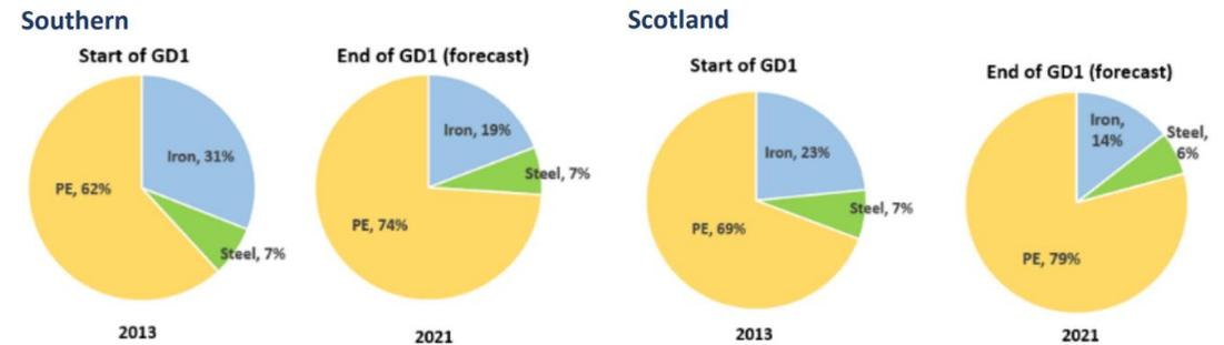
**% of PE mains in gas networks at start and end of GD1 (SGN Network)**
