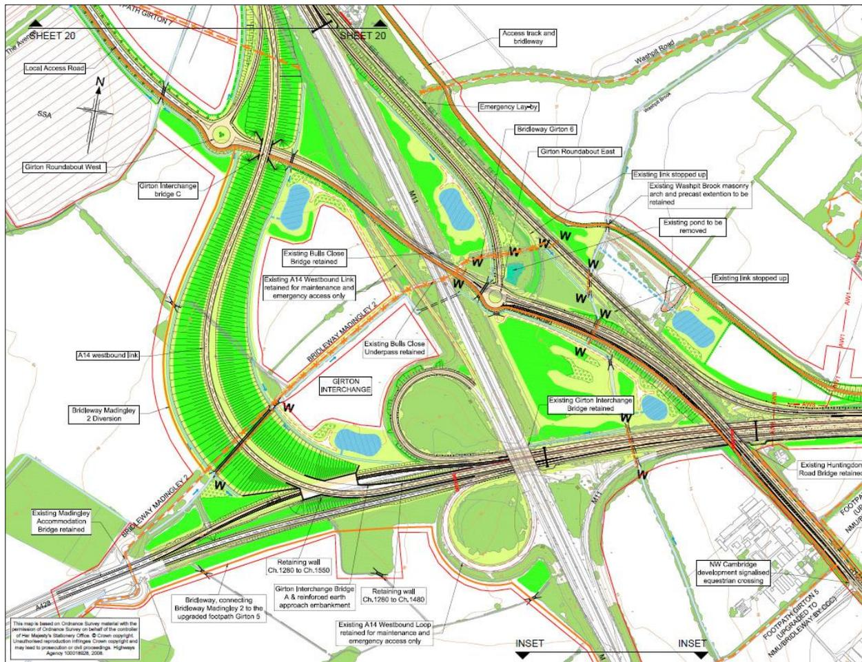
Figure 6: Draft plan of Highways England's remodelling of the Girton Interchange ([download as a PDF](#))
