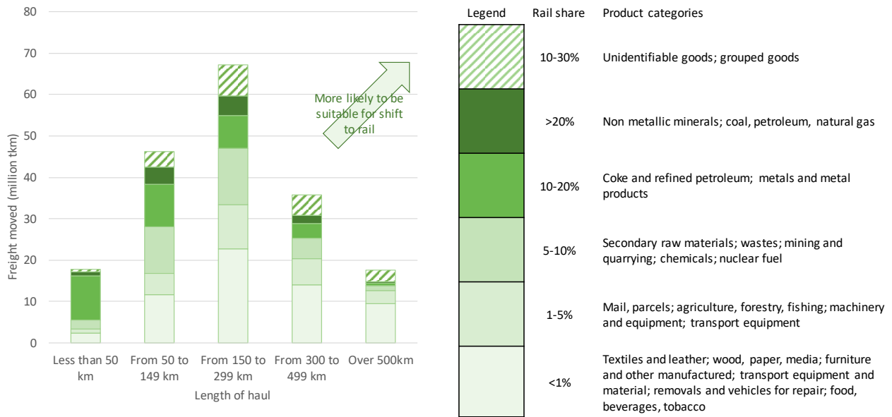
Figure 20. There may be an opportunity to shift from road to rail in some freight market segments
