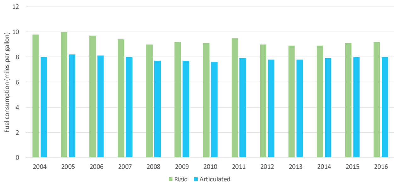
Figure 27. There has been no discernible improvement in the fuel efficiency of HGVs over the last decade
