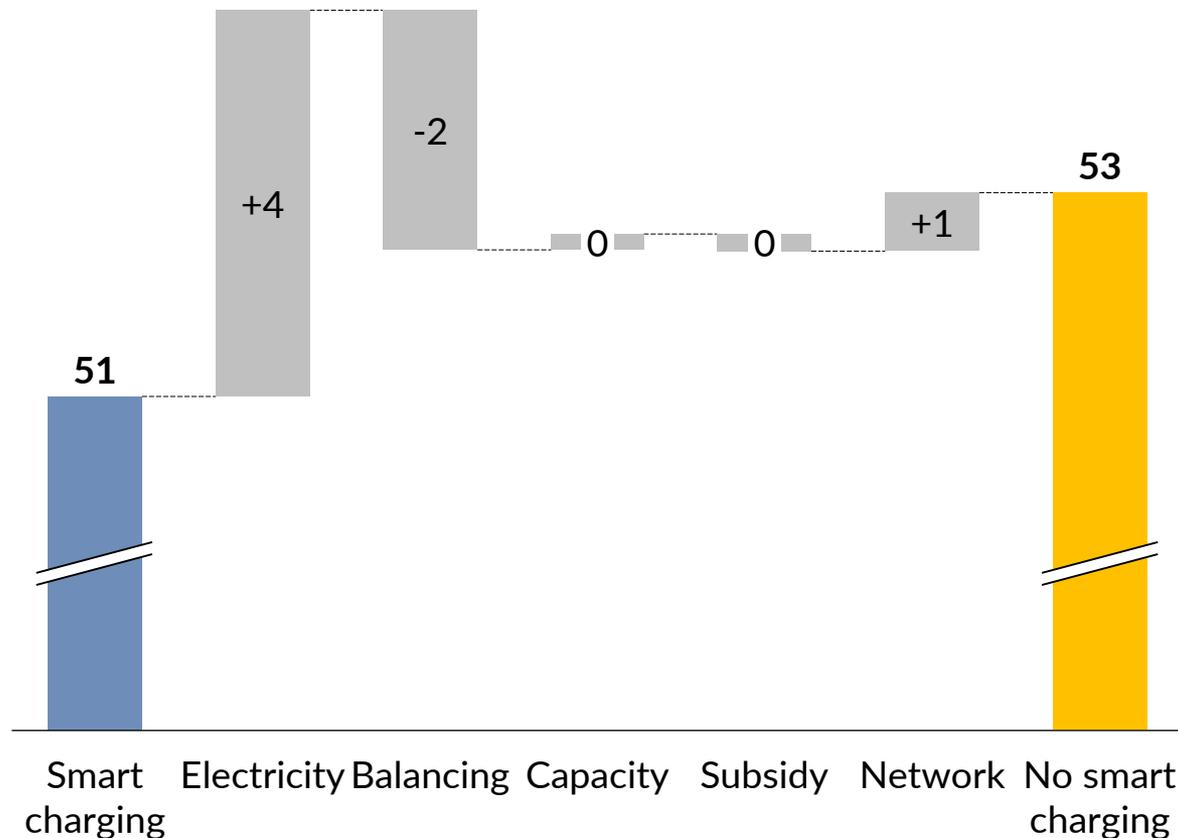
1. Costs have been averaged over all different RES penetrations levels to give a sense of the main drivers of cost increases when moving from smart to not smart charging.
