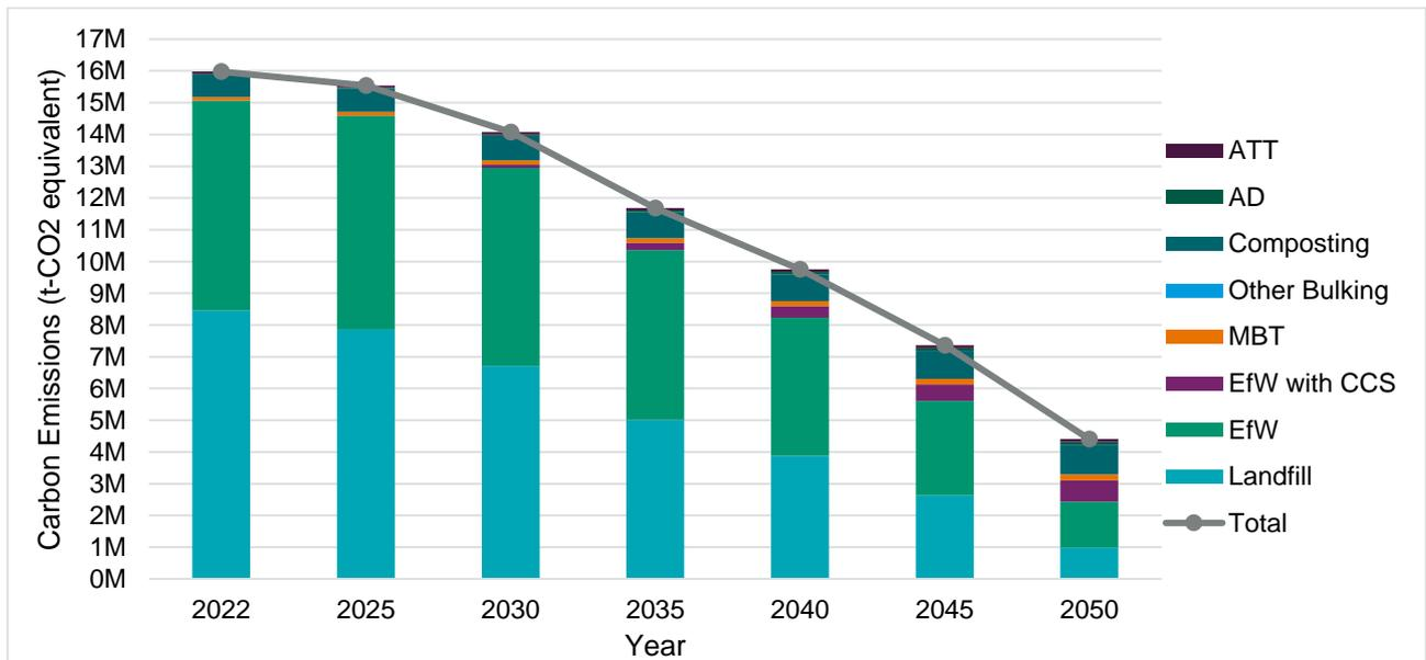
Figure 24: Scenario 4 (Low Composition) Carbon emissions per facility type
