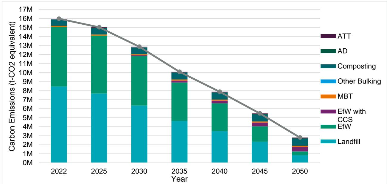
Figure 23: Scenario 3 (High Composition) Carbon emissions per facility type
