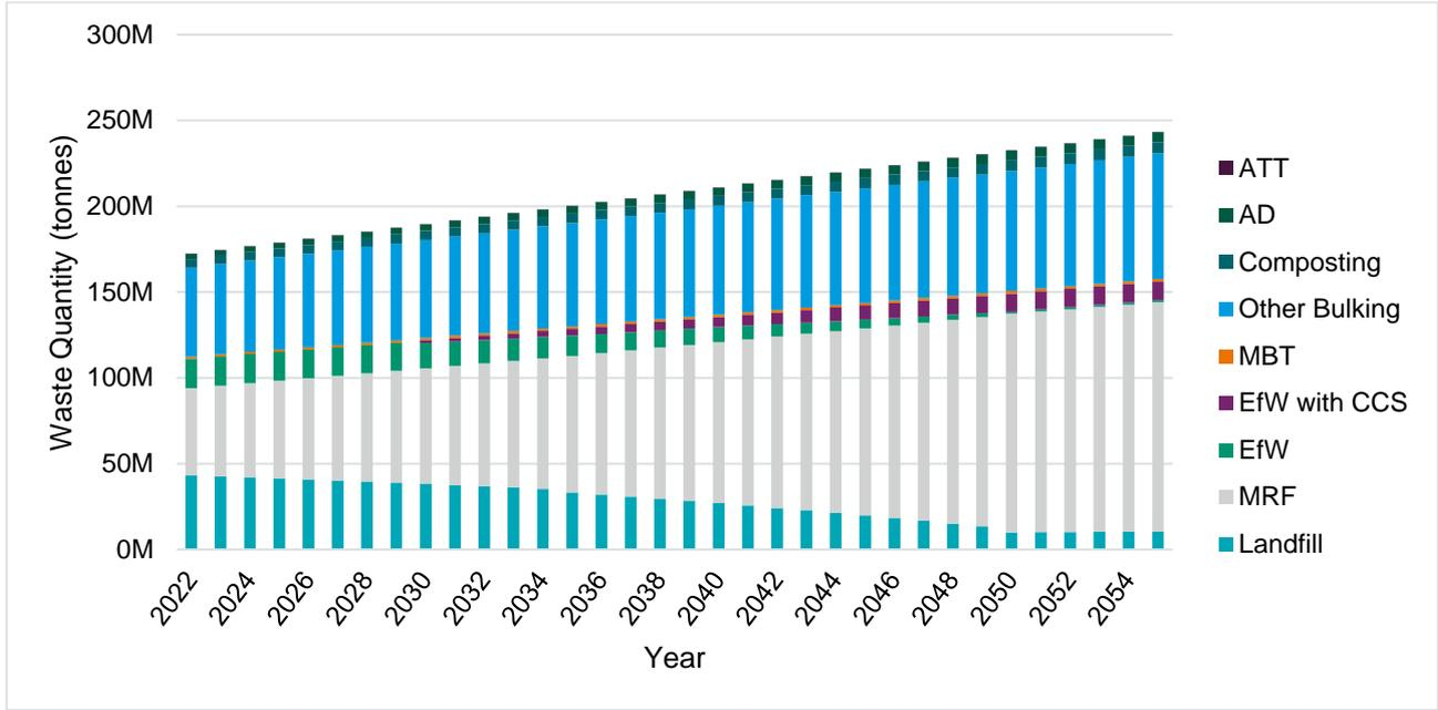
Figure 17: Scenario 2 (Low Arisings) Tonnes per facility type<sup>46</sup>
